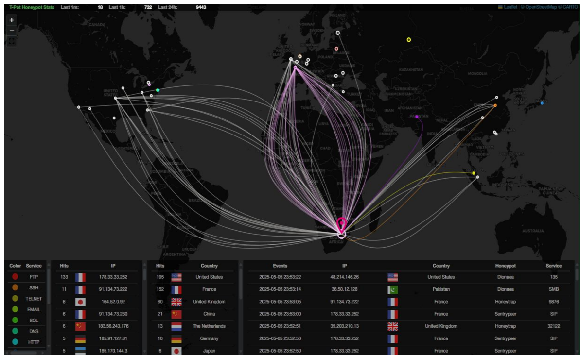
Figure 6: T-Pot attack map showing the geographical distribution of observed attack activity
