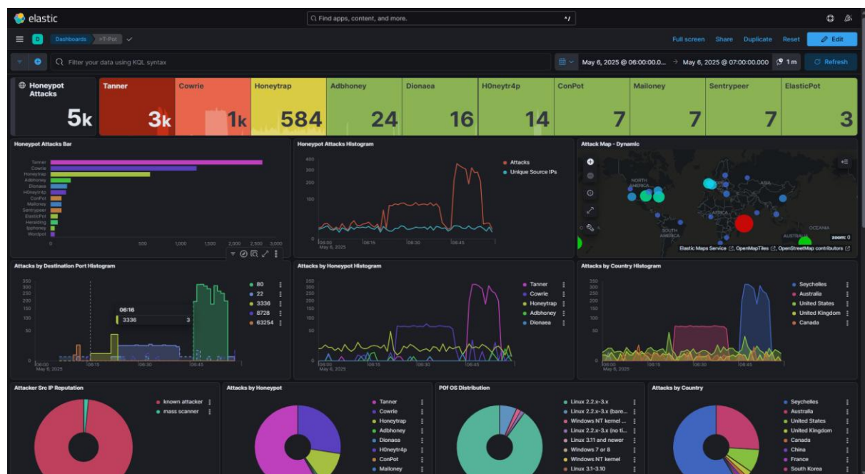
Figure 8: Kibana dashboard showing attack activity involving port 502 during the deployment
