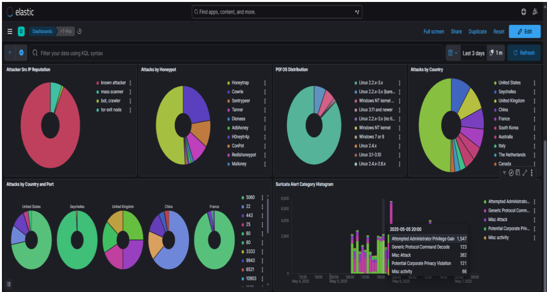
Figure 4: T-Pot visualisations showing attacks by country and port, source-IP reputation, honeypot distribution and operating-system information
